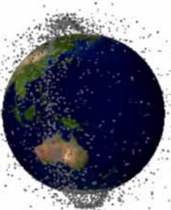
Figure 4: Debris cloud after 6 months.
