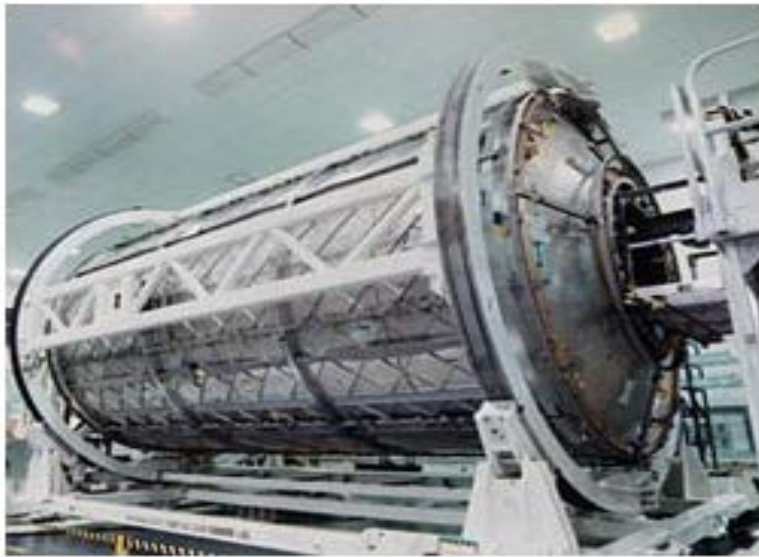
The U.S. Laboratory module for the International Space Station awaiting to be covered by a debris shield blanket.
