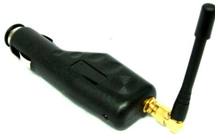
Commercially- available GPS jammer (2014)
