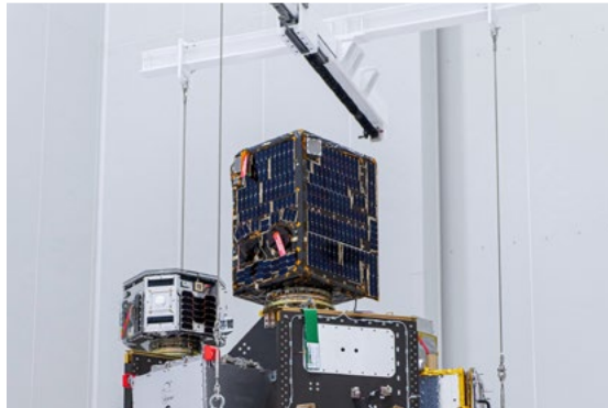
Figure 3.4 | Vega's Small Spacecraft Mission Service dispenser with multiple satellites is lowered onto the rocket's payload adapter at Guiana Space Centre in Kourou, French Guiana in June 2020. Credit: ESA
