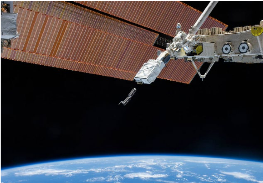
Figure 3.5 | Robotic deployment of satellites, in this figure from the Small Satellite Orbital Deployer (SSOD) held by the ISS's Kibo robotic arm, presents other opportunities to launch satellites into orbit. Credit: NASA
