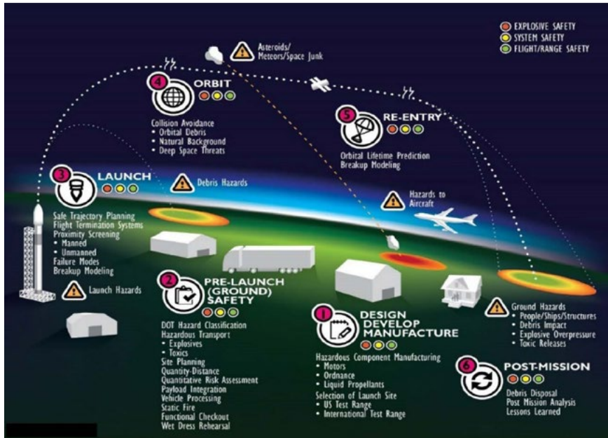
Figure 3.6 | This figure illustrates the typical stages a launch vehicle goes through and the types of safety considerations at each stage. Credit: FAA
