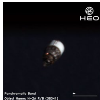
Figure 3.3 | Image of an H-2A rocket body taken by a space-based sensor. Credit: HEO Robotics
