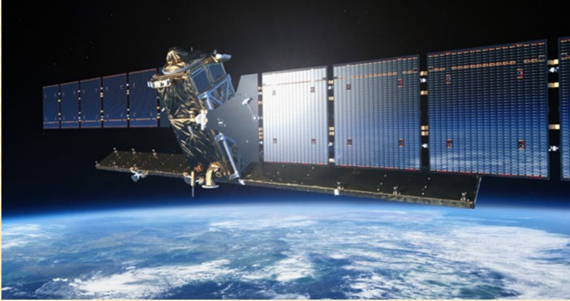
Figure 3.10 | ESA illustration of the Sentinel 1-A C-band Synthetic Aperture Radar (SAR) satellite. Credit: ESA
