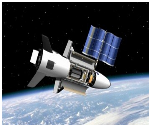
Artist's rendition of how the X-37B will deploy on orbit, including the solar panels used for electrical power. Image credit: Boeing
