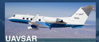
Using an airborne radar to study earth science (earthquakes, volcanoes, vegetation, hydrology, ice, etc.), with emergency response potential
